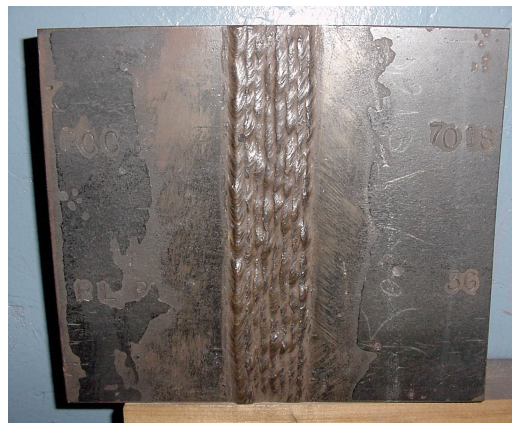
Example of a High Quality Weld
